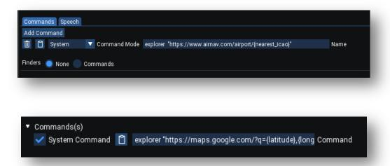
The command format is similar to what you would see if running the command from a DOS box or a unix terminal. The first part is the program to execute and the latter parts are the command arguments. The program must be able to be found in your environment PATH. If it is not then you will need to specify the full path to the executable.
