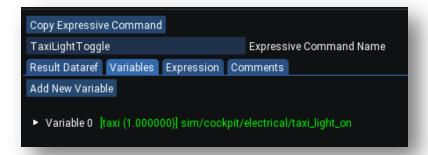
When the key associated with this expressive command is pressed a simple evaluation will be performed and the result will be written to the taxi light dataref. If the taxi light is off then return 1 which will turn it on and if it was not off (meaning it was on) then return 0 which will shut it off.
